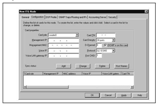
Note 1: The Voice LAN Node IP address on the General tab and the Voice IP and Voice LAN gateway IP addresses for Leader 0 and Leader 1 on the Card Configuration tab must be on the same Voice or T-LAN subnet.
